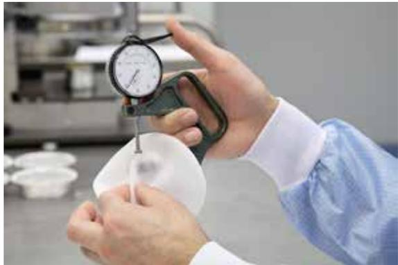
The maximum and minimum shell thickness are ascertained via approximately 10 measurements in three areas: the front (anterior), at the edge (equatorial), and the back (posterior). The results are checked for compliance with the specifications for implant shells. The weight is also an indicator of the thickness and regularity of the shell. Only shells that comply with the specifications proceed to the next step in the production process.
